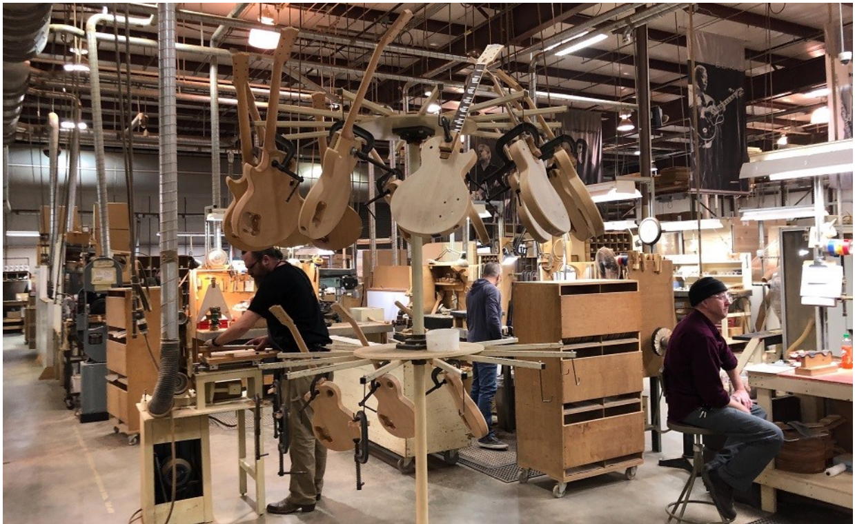
Necks are glued to bodies and air-dried at this station at the Gibson Custom Shop in Nashville.
